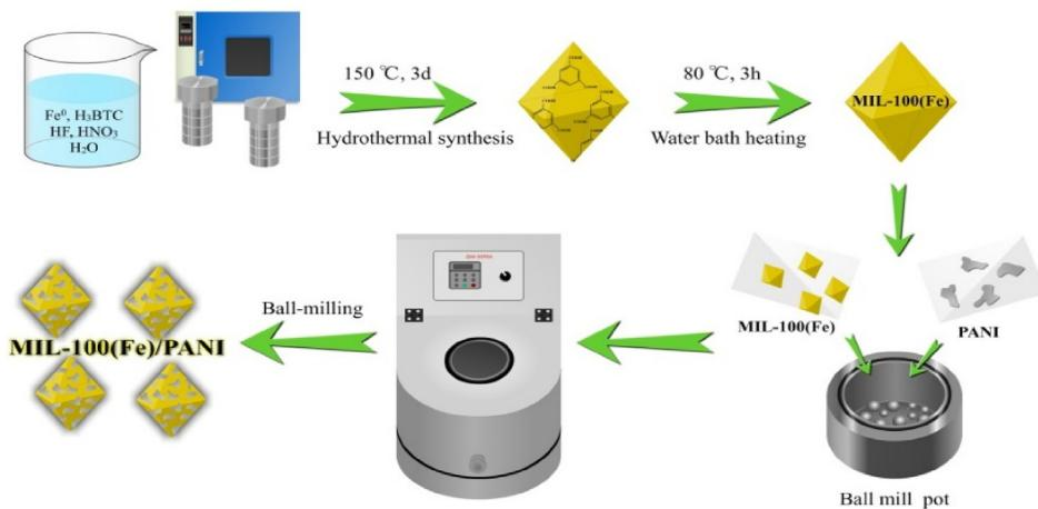
**Scheme 1.** The preparation procedure illustration of MIL-100(Fe)/PANI composites.
